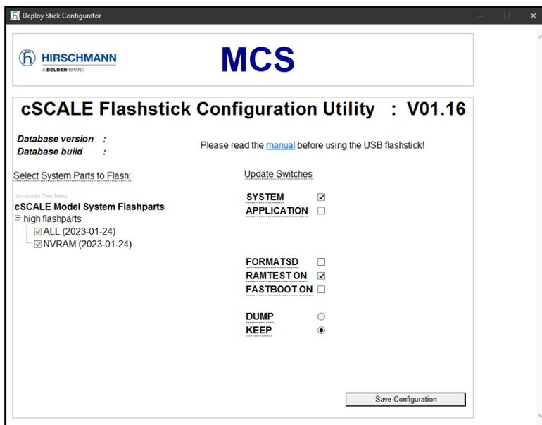
Please make sure that the flash parts boxes “ALL” and “NVRAM” are all checked. Make sure that the update switch is set to SYSTEM. Save the configuration.
