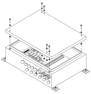
4. Reinstall cover and tighten screws, making sure the rubber gasket, is positioned correctly, to prevent any moisture, from entering the central unit.
