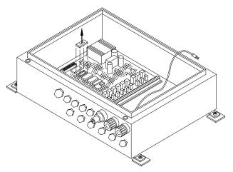
2. <u>CAUTION</u>: Discharge any static electricity, from your body, before handling the EPROM. The EPROM could be damaged, if this procedure, is not followed. Remove the old DATA EPROM, from the main board. Be careful to pull the EPROM out, without bending the legs. Refer to drawing above.
