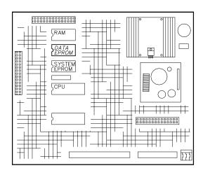
3. Carefully align the new EPROM, with the socket and push the EPROM, into the socket. Be careful not to bend any of the legs. Refer to drawing.
