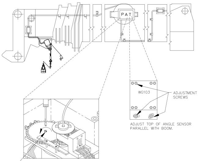
ADJUST LENGTH POTENTIOMETER, WITH BOOM FULLY RETRACTED TURN THE CENTER SCREW COUNTER CLOCKWISE TO A SOFT STOP.
