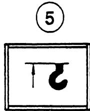
This red warning light (5) will light up when the anti-two-block limit switch contacts open, indicating that a two-blocking condition is approaching. At the same time the audible alarm will sound.
