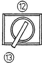
The position (13) by-passes the anti-two-block control lever lock-out which does not influence the LMI system. The red warning light (5) and the audible alarm (16) for approaching two-block condition will also come on at all times. The by-pass key switch is spring-loaded in order to return the switch to the neutral position (14). To activate the switch, it therefore has to be held manually during its operation.
