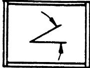
Button (10) activates the features to recognize and work with boom angle limits. After this function has been activated, the lamp in the button will light up and the display will show the max. and min. angle presets in addition to the data for radius, length and actual angle. Once these angles are reached, the horn will sound until the boom is moved back into permissible angle range.
