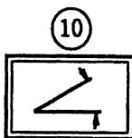
To indicate that the angle limits are activated, the lamp in the button (10) will light up.
