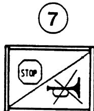
This control (7) serves a dual purpose. First, it is a red warning light, which warns the operator that a rated load condition has been reached. It lights up, when the load on the crane is at 100% of the crane rating. Second, it allows the audible alarm to be silenced for 15 seconds by pressing this button.
