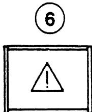
This yellow light (6) will light up when the load on the crane is between 90 and 100% of the crane rating, indicating that an overload condition is approaching.
