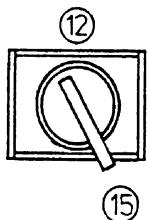
In this position (15), the by-pass key switch (12) deactivates the control lever lockout function of the LMI. All other display, indicating and alarm functions, as well as the control lever lockout function of the anti-two-block system will continue to work. The by-pass switch is springloaded in order to return the switch to the neutral position (14). Therefore to activate the switch, it has to be held manually during its operation.
