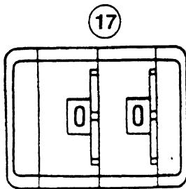
The operator has to set the operating code switches (17) to the determined operating code number.
