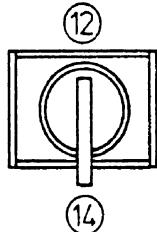
This is the neutral position (14) to which the switch returns because of its spring-loaded mechanism. In this position, the by-pass switch is without influence to the LMI and anti-two-block control lever lock-out.
