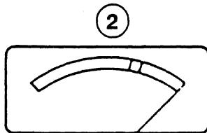
The load moment will be displayed in the indicator (2). This meter displays how much of the crane rated capacity is being used. As the rated capacity of the crane changes as it is moved through its various motions, the meter will constantly change to coincide with the crane ratings.
