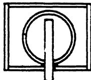
The element (12) is a switch which can only be activated with a key. This by-pass key switch can deactivate the cut-off of the LMI or anti-two-block momentarily to allow the crane operator to override the control lever lockout. The spring-loaded by-pass switch has 3 positions which are further described as follows.
