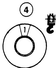
The Reeing Switch (4) provides the load moment indicator with information regarding the number of parts of line used to reeve the hook block. The switch has 16 positions which are shown under the window of the control knob when it is turned.
