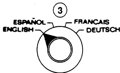
After the ignition of the crane has been activated and the system has passed through the system test without errors, the console will display this phrase alternately in all 4 languages. With the switch (3), the crane operator can select the desired language. The language does not have any influence on the function of the system.
