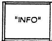
The button (9) is used to request information which will be shown on the display (1). The direction to use this button will be given through the information PUSH "INFO" at the display.
