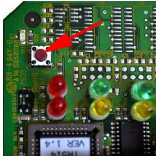
▲ 4. View of the programming button and the LEDs on the circuit board
