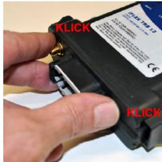
▲ 9. Lock the circuit board by applying strong pressure to the underside of the housing (clearly audible click at both sides).
