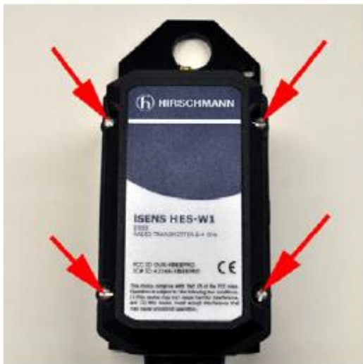
▲ 1. First of all, open the battery compartment of the wireless hoist limit switch to be registered by undoing the cover screws and removing the cover of the battery compartment.
