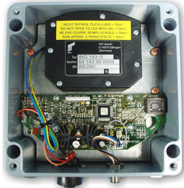
CAN-Bus electronics in angle sensor box.
