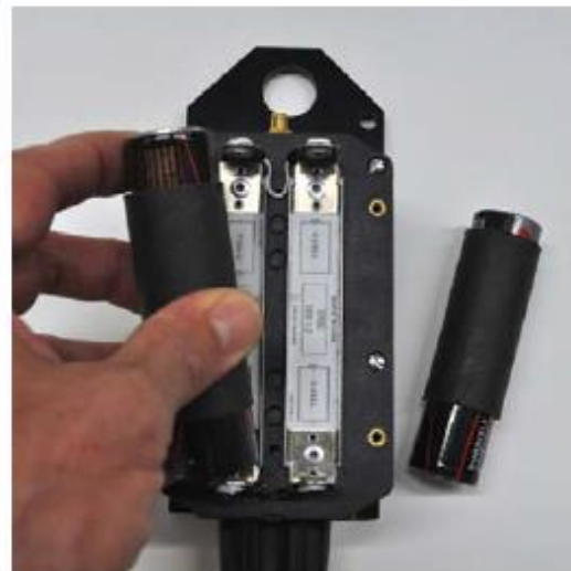
▲ 2. Remove the batteries
