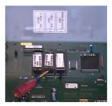
3. Replace I.C. with notch down and flat side to the top as shown in diagram. WARNING: If I. C. is placed in wrong, the I.C. will be destroyed and a new I.C. will have to be ordered.
