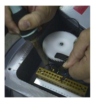
7) Tighten the <u>three mounting screws</u> that hold the angle sensor in place:
