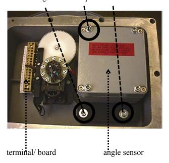
6) Before tightening the angle sensor back in place, make sure that these <u>three wires</u> can move freely and are <u>not pinched</u> between the angle sensor and the mounting:
