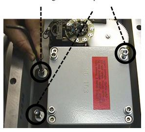
3) If the terminal block looks like this (DS 350 G system): unsolder wires 4, 5, and 6:
